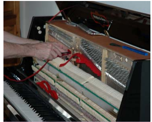
Having opened the piano up Andrew now silences two out of three of the strings on each key which allows him to here each string separately.
